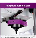
Spindle lock with integrated ejector for easy tool change
